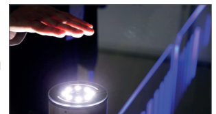
//Touchless 4-fingerprint sensing unit integrated in entry system from WANZL.
