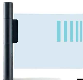
//Touchless 4-fingerprint sensing unit integrated in entry system from WANZL.
